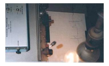
Electrical signals are fed from the electrode assembly, through a shielded cable, to the biological pre-amplifier. The signal from the pre-amplifier is then fed into a recording amplifier which provides a sensitivity control and a pen centering control. The display on of the EEG provides a graphic read-out of the net electrical potential changes from the oral leukocytes being monitored.
