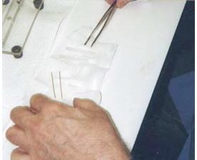
They take two 60 mm. lengths of gold wire, about 1 mm. in diameter, and making sure they are sterile, they insert these little gold electrodes into the culture tube, maintaining careful separation with the use of rubber bands.
