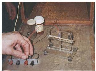
In a screened cage, two flexible wire leads are then attached to the top of the gold electrodes by means of small firmly gripping alligator clips, which are also kept carefully apart. The chart drive is set for EEG sensitivity. [For those who know this stuff, passband frequency settings were for a range of .2 Hz low and 50 Hz. high.] From there we have the copper-screened cage around the culture test tube to block AM or FM signals, and similar cycles of the electromagnetic spectrum.
