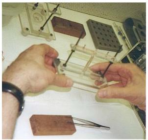
What they are doing is getting the "net electrical potential activity" of the in vitro white cells. Not just a few cells, but millions of them. Through the wire, the electrical signals are fed from the electrode assembly, through a shielded cable, to the biological preamplifier, a type that is suitable for EKG or EEG recordings.
